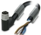
Power cable, 4-position, PUR halogen-free, black-gray RAL 7021, free cable end, on Socket angled M12, coding: T, cable length: 1 m, For direct current up to 12 A/63 V
