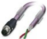
Bus system cable, PROFIBUS (12 Mbps), 2-position, PUR halogen-free, violet RAL 4001, shielded, Plug straight M12 SPEEDCON, coding: B, on free cable end, cable length: Free input (0.2 ... 40.0 m)
