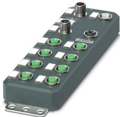
Axioline E, Digital I/O device, PROFIBUS DP, M12 fast connection technology, Digital inputs: 8, 24 V DC, connection method: 4-conductor, Digital outputs: 4, 24 V DC, 2 A, connection method: 3-conductor, Plastic housing, degree of protection: IP65/IP67
