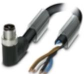
Power cable, 4-position, PUR halogen-free, black-gray RAL 7021, Plug angled M12, coding: T, on free cable end, cable length: 1 m, For direct current up to 12 A/63 V
